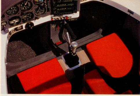
A bicycle-type brake handle is mounted on the stick. The throttle is positioned high on the left side.
